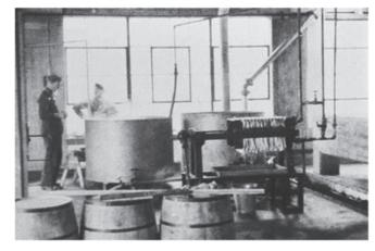
Fig. 2 Citric acid fermentation at Pfizer's Brooklyn facility during 1920s
